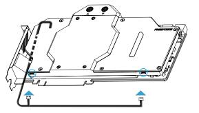
Connect the 2 RGB connectors to the RGB LED strips.
