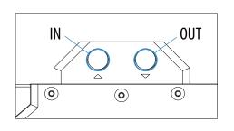
Screw in the two G1/4 threaded male fittings, attach the liquid cooling tubes and connect the water block(s) into the cooling circuit. Phanteks recommends using Phanteks fitting with the Phanteks Glacier Series water blocks.
