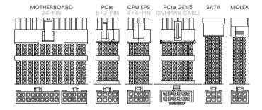
Connect the cables to the Revolt power supply:
